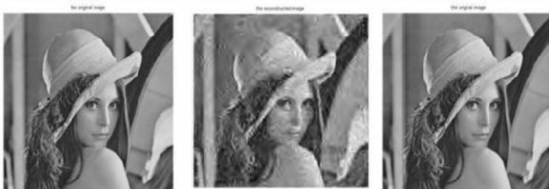
Fig. 2: The decoded LENA image from left to right, (a) original, (b) original OFDM [PSNR= 24.5140 dB], (c) modified OFDM (UEP ) [PSNR= 30.4160 dB]
